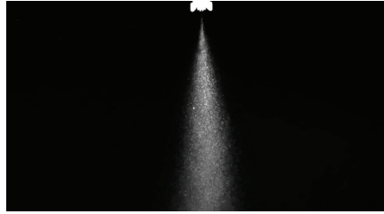
Polyacetal construction provides a wear resistant orifice to ensure pattern integrity.
