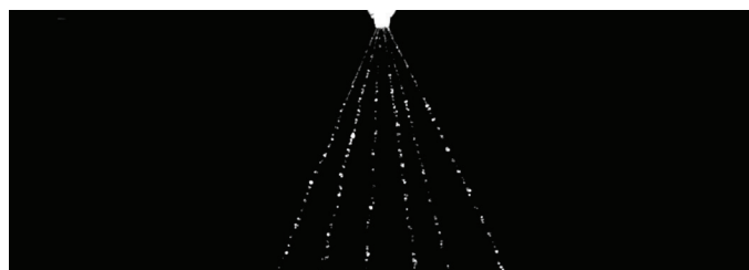
110° wide pattern consisting of 6 equally spaced streams providing uniform deposition of liquid fertilizers. Each individual stream was engineered to hold stream integrity and not break apart to avoid unwanted fertilizer burn on post emerge applications.
